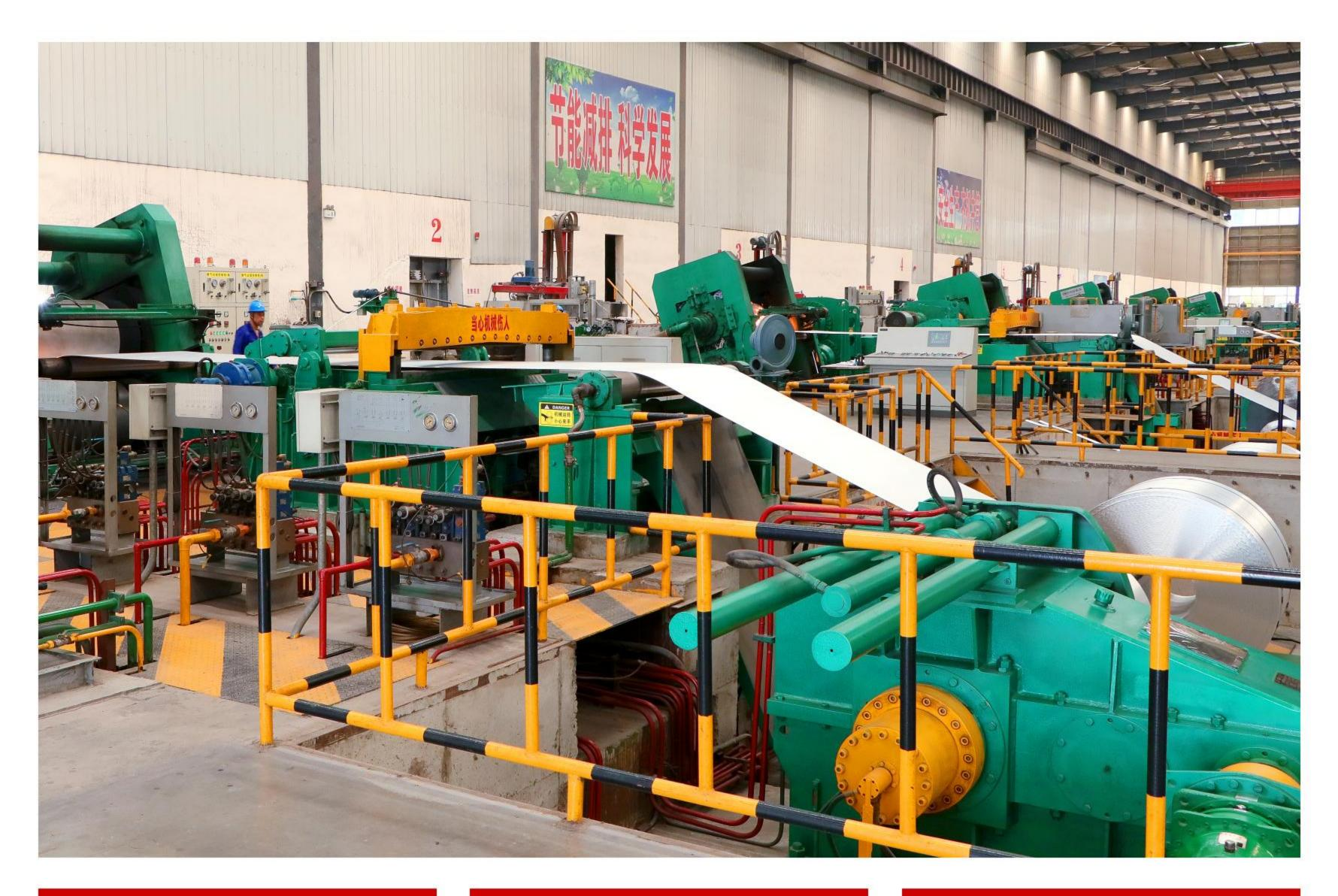
Roll diameter φ600~φ1200mm Rolling speed 800~1500mm/min
